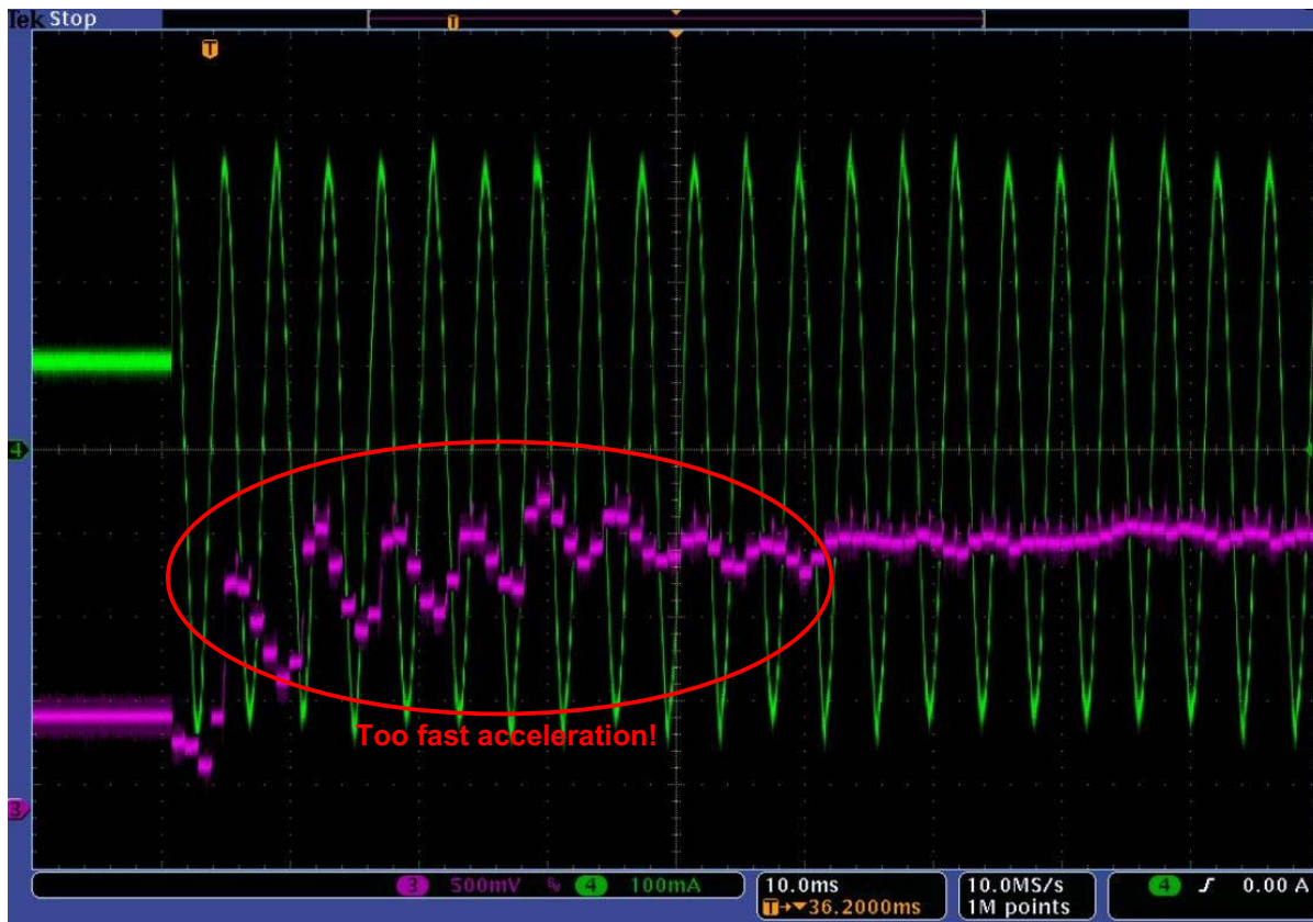
Figure 34. Too Fast Acceleration Results in Overshoots
